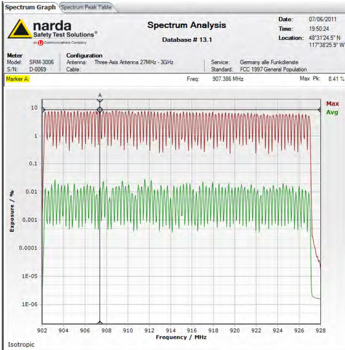
Figure 3-2 Example SRM-3006 spectrum measurement of the spread-spectrum frequency-hopping signals produced by a L+G Focus AXR-SD smart meter at 0.3 m showing the 83 hopping channels used by the meter. The marker is set on the maximum peak value of field representing 8.41% of the FCC MPE for the general public.
